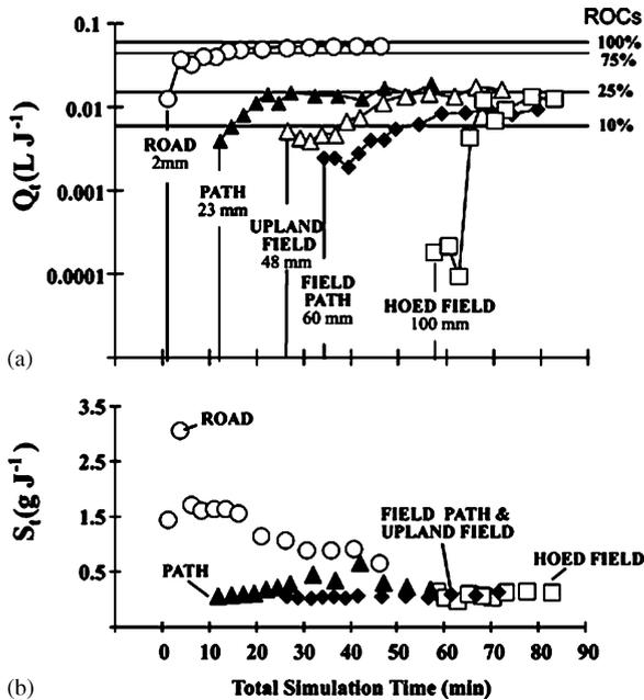
Fig. 7. (a) Energy-normalized instantaneous discharge ( $Q_t$ ), runoff coefficients (ROCs, %), and rainfall depth (mm) before runoff generation for several land-use types in PKEW during rainfall simulations; (b) normalized sediment output ( $S_t$ ) during the same simulations. Data and simulation experiments are described in detail elsewhere (Ziegler et al., 2000b).
