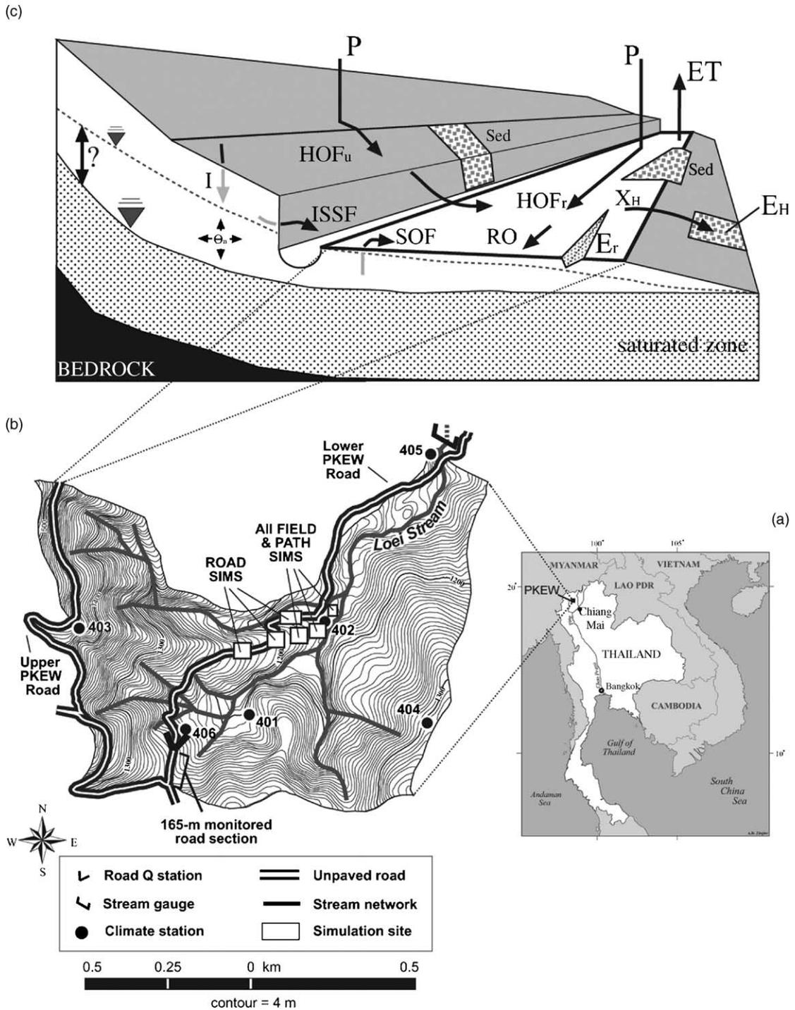
Fig. 2. (a) Pang Khum Experimental Watershed (PKEW) in northern Thailand; (b) experiment locations in the 93.7 ha PKEW; the climate network and simulation sites are explained briefly in Sections 4.2 and 4.3; (c) conceptualization of important processes operating on the three-dimensional road prism. Abbreviations are defined in Section 3.
