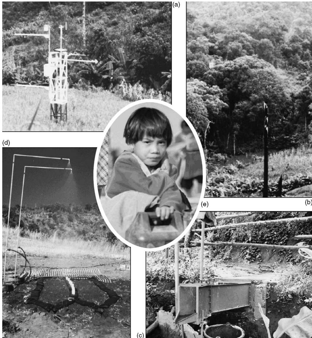
Fig. 4. (a) Climate station 402, in an upland rice field (see Fig. 2b for station location); (b) climate station 401, above the canopy of a 20 m disturbed primary forest; (c) flume at the road collection station near Station 406; (d) rainfall simulator and plot layout on an upland field, ca. 1998; (e) Lisu girl collecting water.
