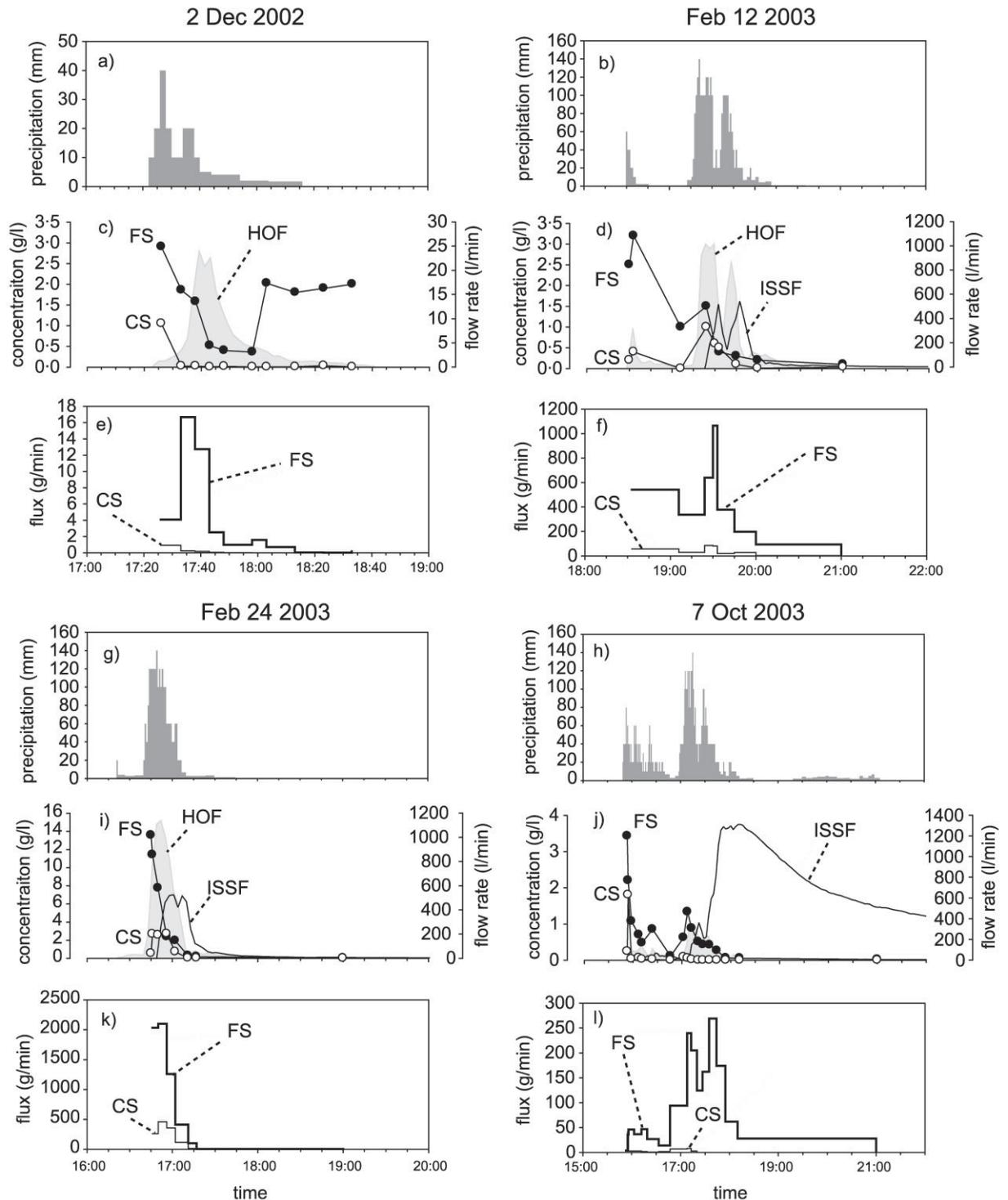
**Figure 8.** For storms on 2 December 2002, 12 February, 24 February and 7 October 2003 the following measurements are shown: (a), (b), (g), (h) precipitation; (c), (d), (i), (j) HOF- and ISSF-related flow rate and sediment concentration for road runoff; (e), (f), (k), (l) flux of coarse ( $\geq 250 \mu\text{m}$ , CS) and fine ( $< 250 \mu\text{m}$ , FS) sediment. All discharge and sediment data are from road weir B.
