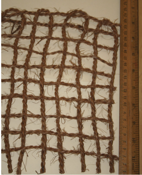
Fig. 2. Open weave coir system with ‘low’ mass per unit area and ‘low’ surface cover (OWCL) (photograph by Laura Sutherland).
