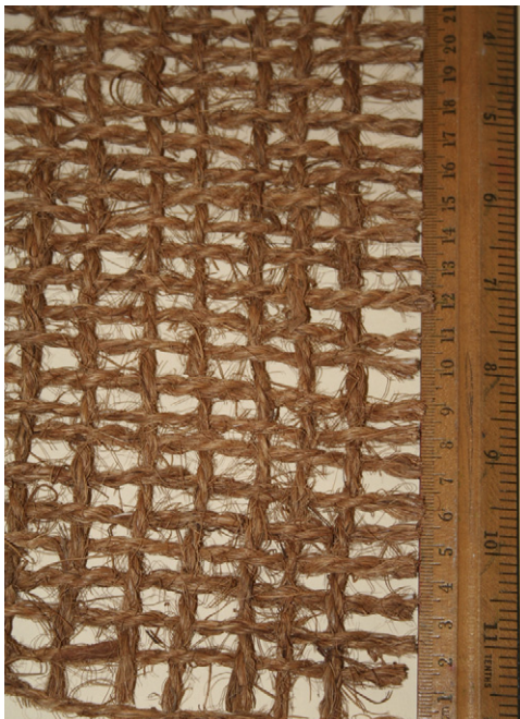
Fig. 3. Open weave coir system with ‘high’ mass per unit area and ‘high’ surface cover (OWCH) (photograph by Laura Sutherland).
