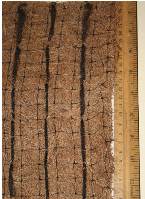
Fig. 1. Random fiber coir (RFC) rolled erosion control system used in this study (photograph by Laura Sutherland).
