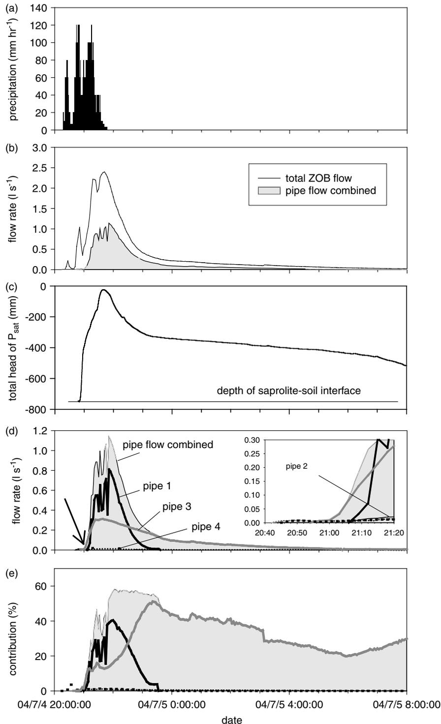
Figure 5. (a) Precipitation, (b) responses of total ZOB flow and combined pipe flow, (c) response of total head of  $P_{\text{sat}}$ , (d) responses of individual pipes, and (e) contribution of pipe flow during the event on 4 July 2004 (76 mm precipitation,  $API_7 = 0$  mm,  $I_{\text{max}10} = 104$  mm h<sup>-1</sup>). Note that the legend of (e) is as (d). The inset in (d) shows an enlargement of the initial flow response denoted by the arrow
