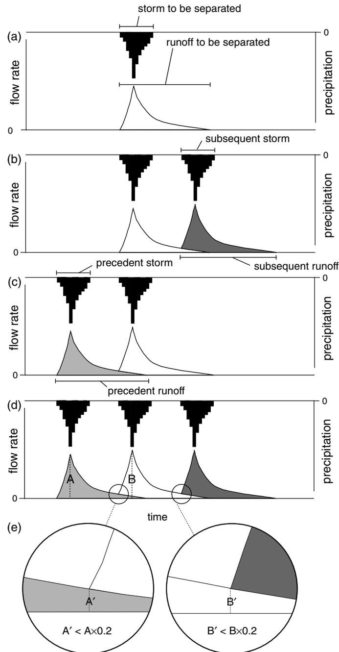
Figure 2. Schematic diagrams showing four cases of ZOB flow separation: (a) case 1, (b) case 2, (c) case 3, (d) case 4, and (e) shows hydrograph separation criteria for multi-event cases. See the text details about each of the cases
