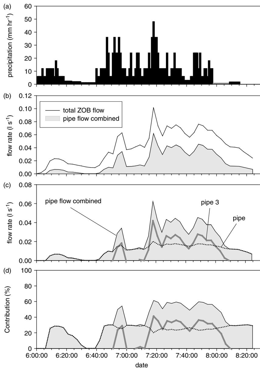
Figure 4. (a) Precipitation, (b) responses of total ZOB flow and combined pipe flow, (c) responses of individual pipes, and (d) contribution of pipe flow during the event on 31 August 2004 (25.4 mm precipitation, API<sub>7</sub> = 6.6 mm,  $I_{\max 10}$  = 25.2 mm h<sup>-1</sup>). Note that the legend of (d) is as (c)
