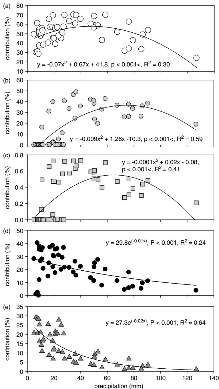
Figure 8. Event-based contributions of (a) four pipes combined, (b) pipe 1, (c) pipe 2, (d) pipe 3, and (e) pipe 4. Note that the relationships in (a), (b) and (c) are polynomial models; the relationships in (d) and (e) are exponential decay models
