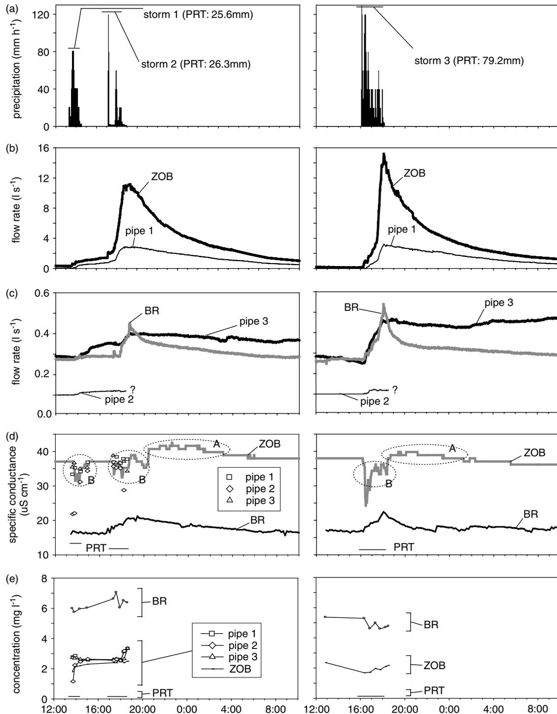
Figure 11. (a) Precipitation, (b) flow rate of the ZOB and pipe 1, (c) flow rate of pipes 2 and 3 and BR, (d) specific conductance, and (e) silicon concentration from various sources (ZOB, soil pipes, and bedrock (BR)) for three storms in November 2004. PRT is event precipitation. Note that data for pipe 4 are not shown because monitoring was terminated in May 2004. Missing flow response of pipe 2 was caused by shortage of data storage in monitoring instruments
