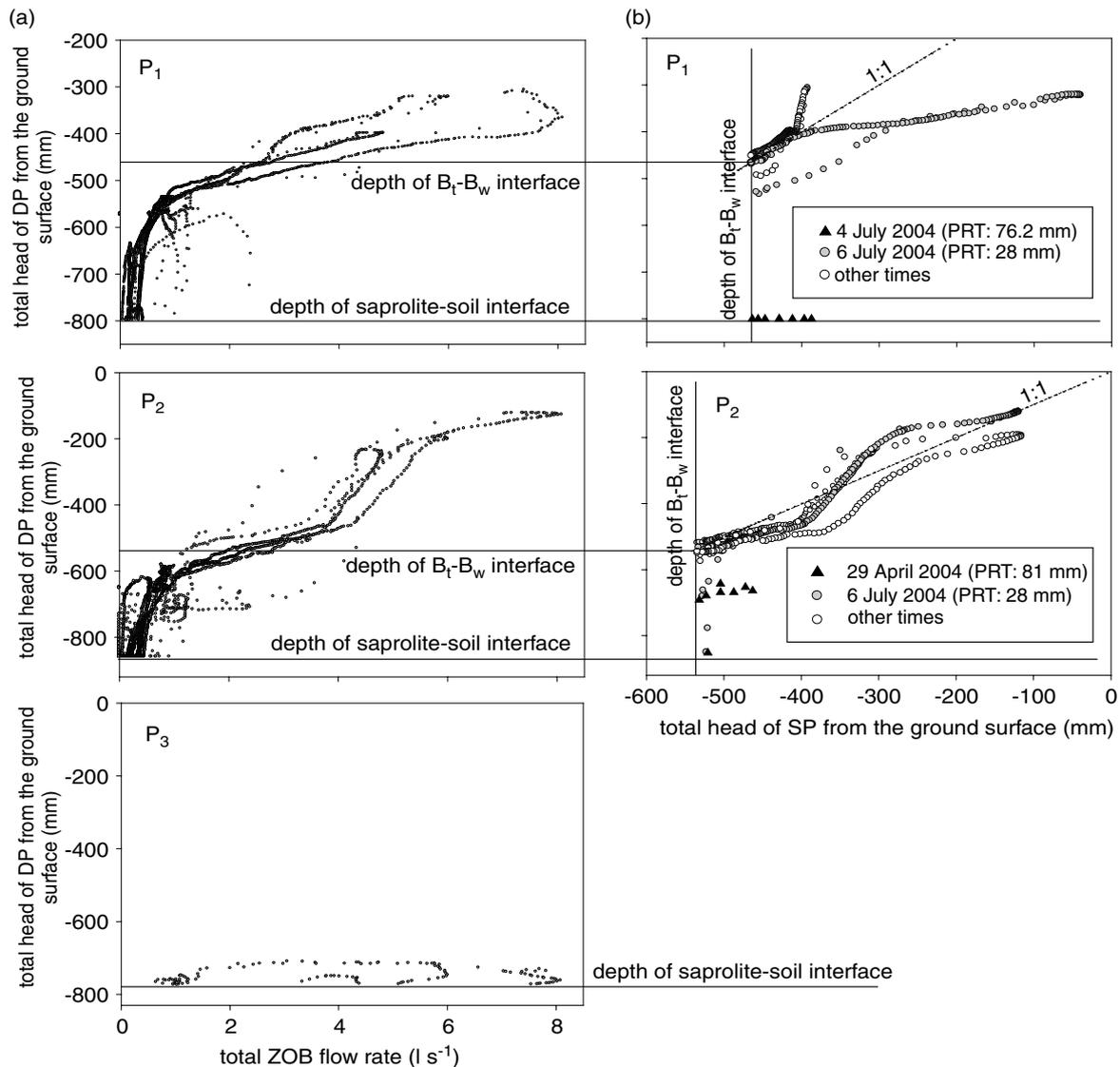
Figure 9. (a) Responses of deep piezometers relative to total ZOB flow. (b) Responses of SP relative to deep piezometer (DP); dotted 1:1 lines predict the relationship between SP and DP when responses of SP are caused by rising of saturated zone detected by DP. PRT is event precipitation
