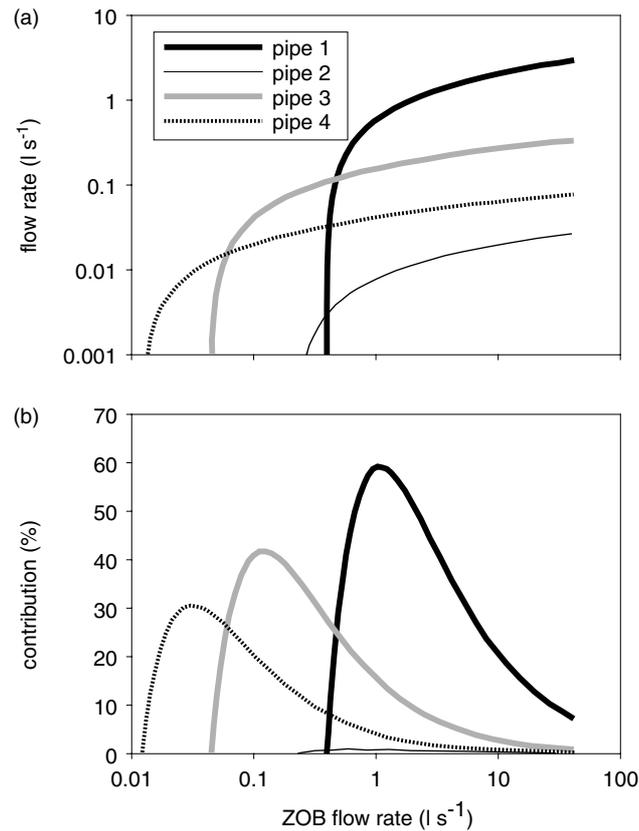
Figure 7. (a) Logarithmic models that relate total ZOB flow rate to flow rate of individual pipes, which were derived from monitoring of pipe flow rate during the study period; see Table IV for the model details. (b) Contribution of individual pipes to total ZOB flow rate. Note that  $x$ -axes on both panels and  $y$ -axis in (a) are logarithmic scales
