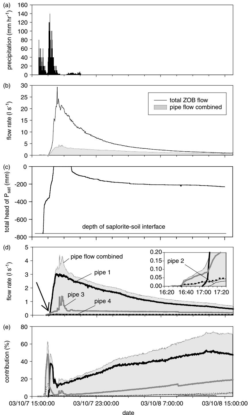
Figure 6. (a) Precipitation, (b) responses of total ZOB flow and combined pipe flow, (c) response of total head of  $P_{\text{sat}}$ , (d) responses of individual pipes, and (e) contribution of pipe flow during the event on 7 October 2003 (86 mm precipitation,  $API_7 = 32.3$  mm,  $I_{\text{max}10} = 110$  mm  $\text{h}^{-1}$ ). Note that the legend of (e) is as (d). The inset in (d) shows an enlargement of the initial flow response denoted by the arrow
