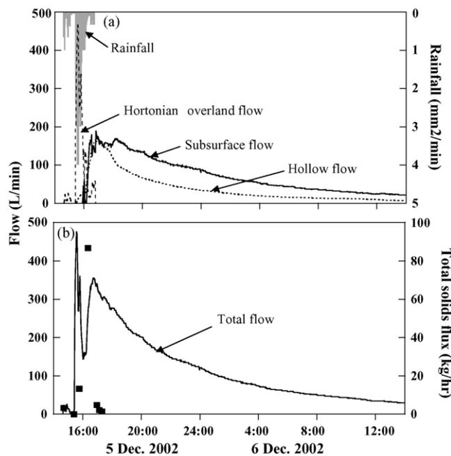
Fig. 6. (a) Separation of road runoff into Hortonian overland flow, intercepted subsurface flow, and flow intercepted from a truncated geomorphic hollow, during a major storm event on 5 December 2002, Bukit Tarek Catchment C3, Malaysia. (b) Composite road runoff hydrograph for the 5 December storm together with measured fluxes of total solids.
