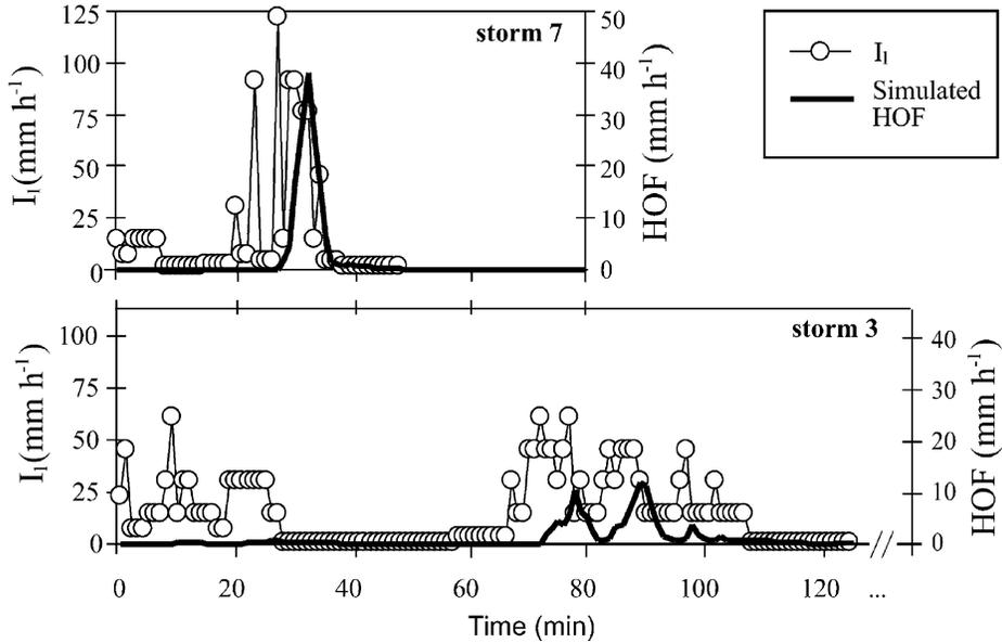
Fig. 8. Comparison of one-minute rainfall intensity ( $I_1$ ) and Horton overland flow (HOF) for storms 7 and 3 (Table 5). HOF is simulated for a 30 × 30 m abandoned field at one-min time steps using the KINEROS2 runoff model.
