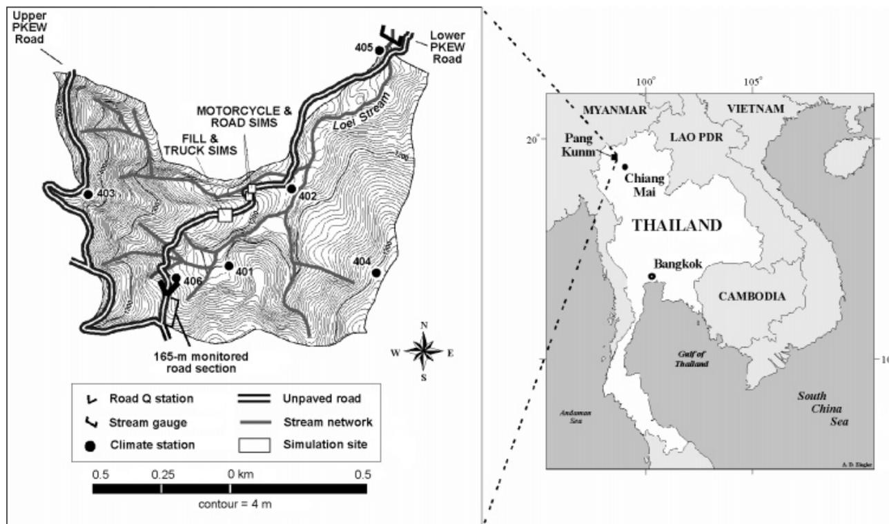
Figure 1. The 93.7 ha Pang Khum Experimental Watershed (PKEW) in northern Thailand. Experiments were performed on the 1650 m section of the Lower PKEW Road bisecting the watershed
