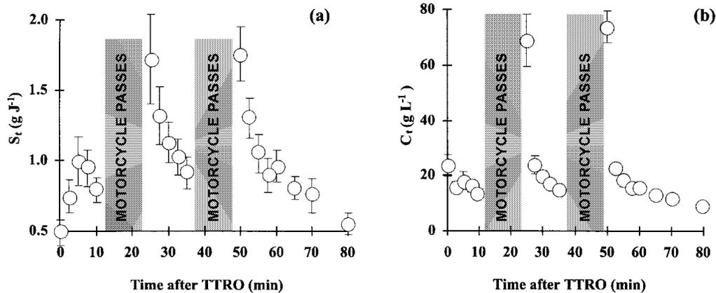
Figure 5. (a) Normalized instantaneous sediment output ( $S_t$ ) and (b) instantaneous sediment concentration ( $C_t$ ) for the pre-pass and two post-pass phases of the MOTORCYCLE simulations. Rainfall was stopped for 15 min to make the motorcycle passes. Each phase time series begins when runoff was generated. Values are means  $\pm$  one standard error
