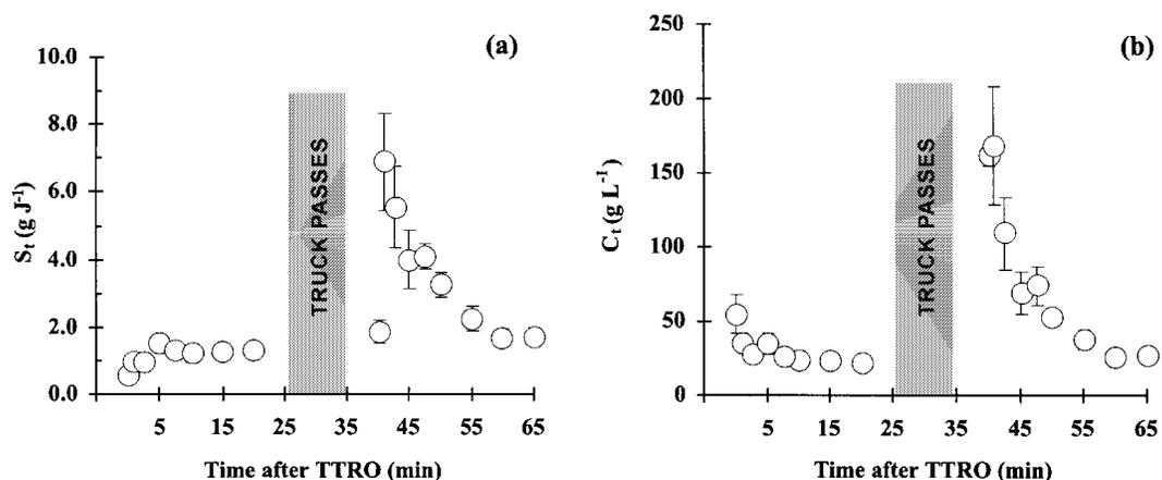
Figure 6. (a) Normalized instantaneous sediment output ( $S_t$ ) and (b) instantaneous sediment concentration ( $C_t$ ) for the pre-pass and post-pass phases of the TRUCK simulations. Rainfall was stopped for 10 min to make the truck passes. Each phase time series begins when runoff was generated. Values are means  $\pm$  one standard error
