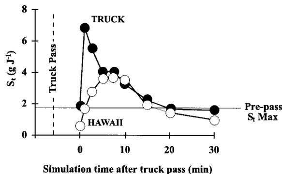
Figure 9. Comparison of post-pass instantaneous sediment transport ( $S_t$ ) for the TRUCK simulations (reported herein) and a previous study in Hawaii (A. D. Ziegler, unpublished data). In both experiments, post-pass values decrease to approximately the pre-pass maximum value after about 20 min (33 and 40 mm of rainfall for the Hawaii and Thailand simulation, respectively)
