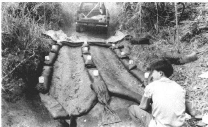
Figure 3. Rainfall simulation plot design shown during one simulation. The bases of the vertical simulator risers rest on the elevated bench to the right of the two subplots. White bottles are used for measuring rainfall intensity. Water flows from the plots into shallow collection trenches at the plot outlet
