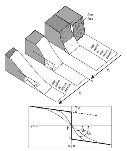
Figure 12 Diagram showing parameters used in the model for slope degradation over time. Note that the vertical coordinate "y" in this figure and in Equation 3, is the same as the vertical coordinate "z" in Equations 1 and 2.
