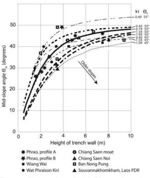
Figure 11 Plot of earthen wall height (h) vs. maximum slope angle  $\theta_m$ . Various curves use different values of  $\theta_0$  and  $k\tau$ , with the heavy line showing the best fit of the data for  $\theta_0 = 50^\circ$ , and  $k\tau = 0.796$ , according to Equation 5 in the appendix.
